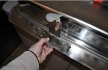
While still supporting the axle in one hand, remove the stabilizer bar, and set aside. Then remove the rolled-cartridge axle.
