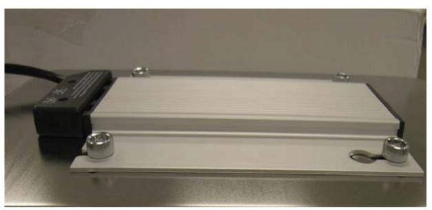
Again, the heating element must be flush with the water pan – you should not see any gaps between the element and the pan. If there is a gap, ensure the bolts are tight. If a gap still remains after you have tightened the bolts, you may have a warped water pan.
